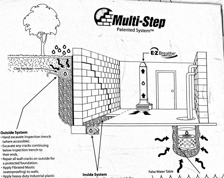
Apply heavy-duty industrial plastic to mastic forming "J" channel.
